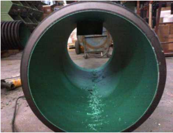
Cut the seal in case it leans into the pipe
